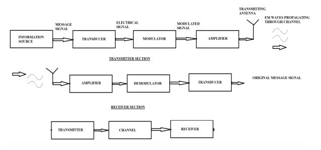
**Information Source:** It is used to generate message signal which may be in the form of audio, video or data.
